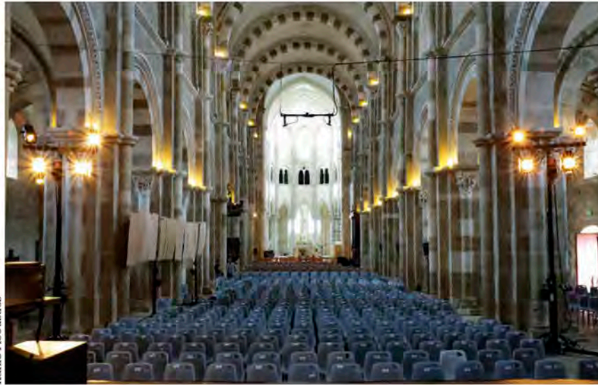
Above: Mock-up testing of mobile reflector panels in the Basilica of Vézelay, France. In this arrangement, the panels are used to enhance sound projection from the stage to the audience
